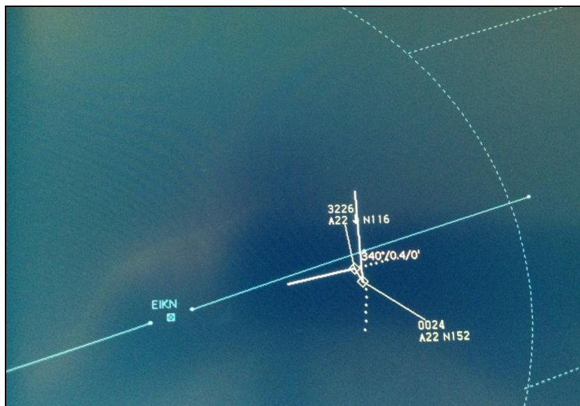
Graphic No. 1: Radar return at minimum separation
